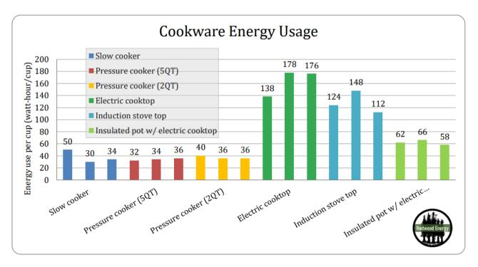
Figure 36: The results of the low power cooking study, the lowest energy use per cup were the pressure cooker and slow cookers.
