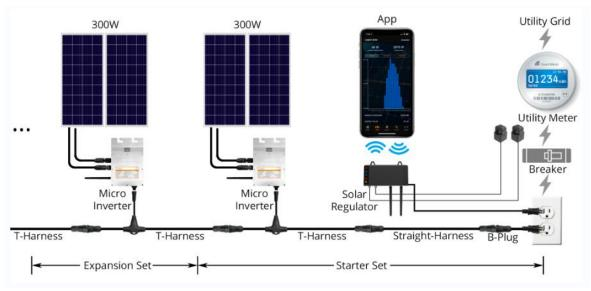
300W and can expand in stages of 300W depending on your budget and needs. Once your system is large enough to have excess energy to store during daylight, you can add expansion sets for nighttime consumption, this expansion set enables the solar panels to charge the batteries, solar panels to supply power to the micro inverters, and batteries to supply power to the micro inverters. No permit needed, plugs in the wall, solar alternative to a backup generator, and a bill saver.
