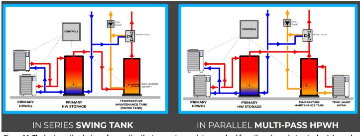
Figure 14: The best practice designs of separating the temperature maintenance load from the primary hot water load. Image by Ecotope.<sup>49</sup>
