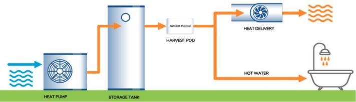
Figure 28: A simple diagram of the Harvest Thermal system.<sup>88</sup>
