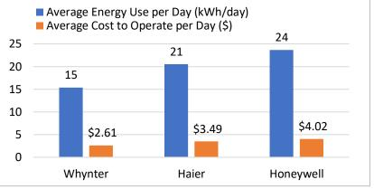
Figure 34: Test results comparing three leading brands of portable heat pumps, tested for a few weeks in Arcata, CA during February-March.
