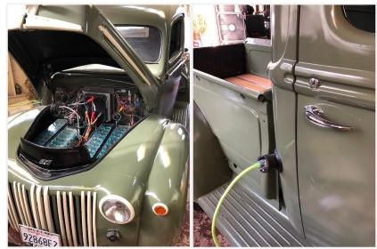
Figure 38: Electrified 1946 Fork Pickup truck.<sup>121</sup>
