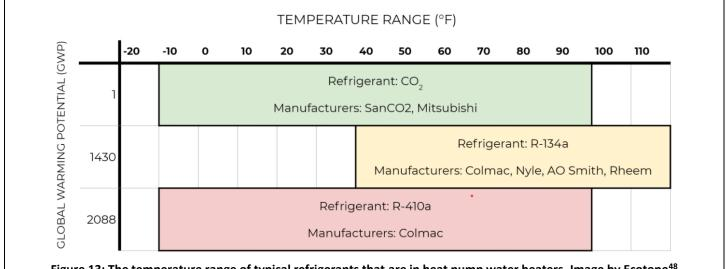
Figure 13: The temperature range of typical refrigerants that are in heat pump water heaters. Image by Ecotope<sup>48</sup>
