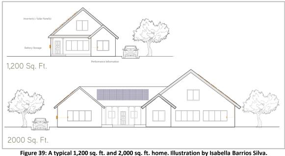
the solar array will be about 200 square feet and 4 kW of DC power. For an average 2,000 square foot house, the solar array will be about 400 square feet and about 8 kW of DC power. Each panel is about 20 square feet and about 400 Watts per panel. To power an average electric car for a year (12,000 miles), it requires an additional 2 kW solar array using 100 square feet of roof space.
