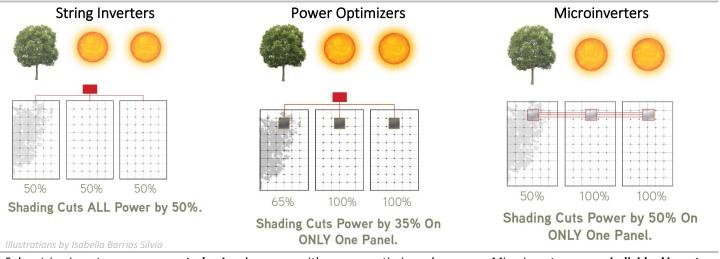
Solar string inverters use **one central inverter** connected to all solar panels in a **single circuit**, such that one panel's shading affects the power produced by all panels. The circuit may have multiple wired ("strings") connecting the panels.
