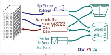
Figure 10: The energy transfer of a condenser water TIER system, as outlined in Taylor Engineering ASHRAE article.<sup>34</sup> (TES = thermal energy storage)
