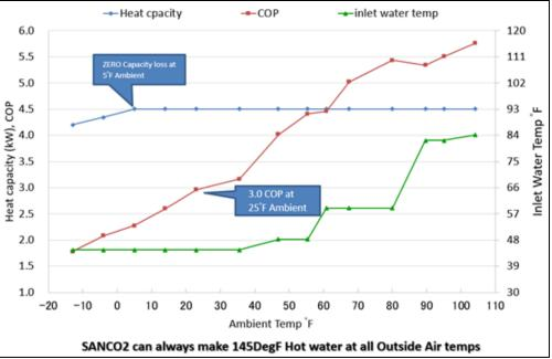
Figure 27: Eco2 heat pump water heater heating capacity, COP, and inlet water temperatures at various ambient air temperatures.<sup>87</sup>
